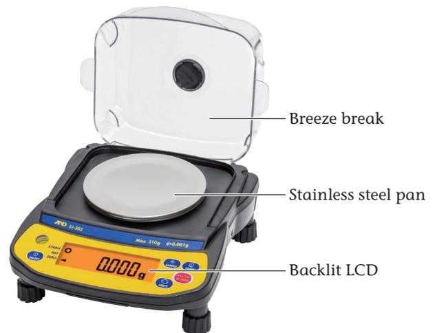
\*<sup>1</sup> Method most commonly adopted for balances with resolutions of one over several hundred thousand or higher. It determines a mass from the amount of current required to generate the electromagnetic force on one side of a lever that equalizes with the mass placed on the other side.
